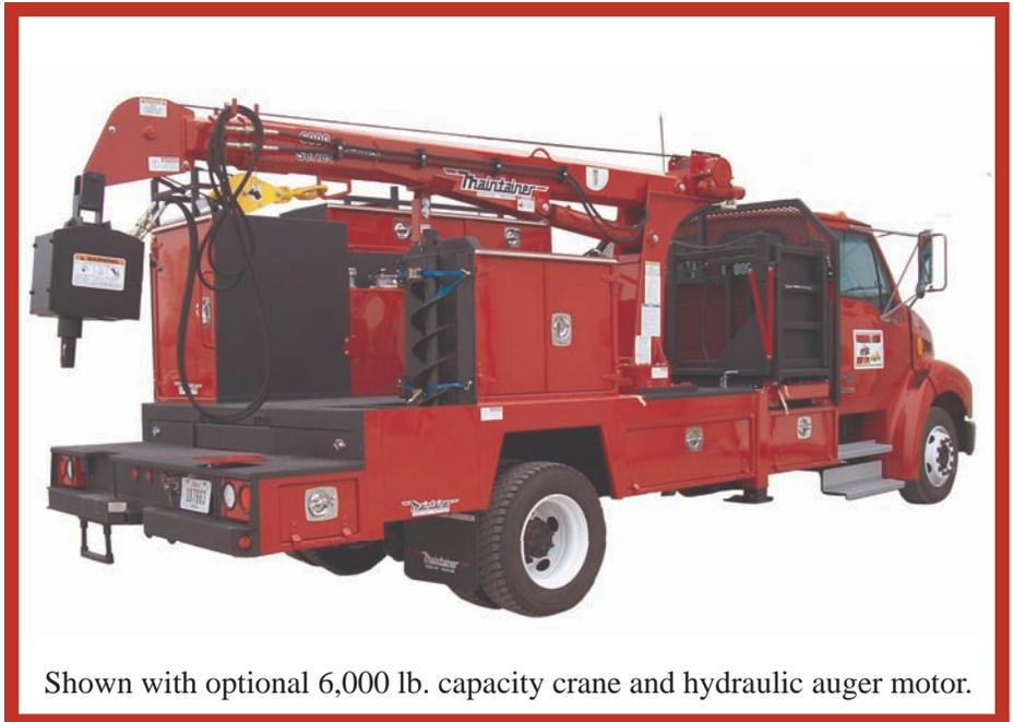
Shown with optional 6,000 lb. capacity crane and hydraulic auger motor.
