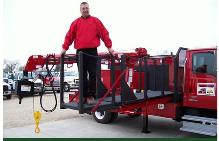
Walk ways were desinged to keep the worker working safely and out of harms way.
