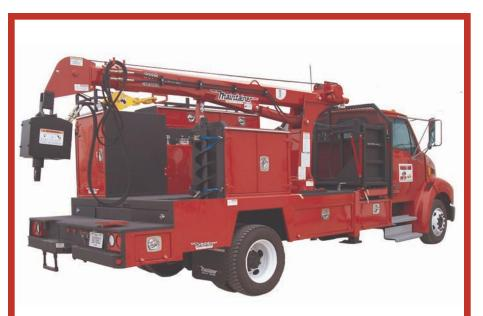
Shown with optional 6,000 lb. capacity crane and hydraulic auger motor.
