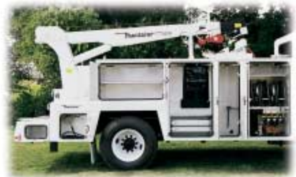
MTSL1 (1-ton service/lube body)
